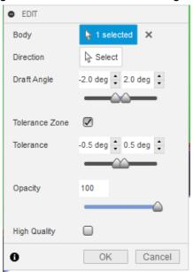
The recommended minimum draft angle is  $2^{\circ}$ , but for secure moulds, we advise using  $4^{\circ}$ . Surfaces without a demolding angle are **highlighted in red, indicating that demolding is impossible.**
