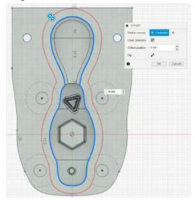
Using the extrusion function to cut both bodies symmetrically about a 0.3mm whole length.
