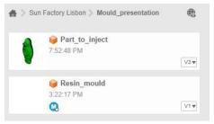
The 3D model used for the mould cavity is imported by drag and drop into the "Resin\_mould" file, creating a link between the two files.
