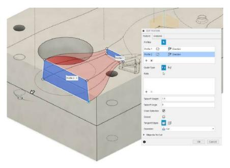
Using the <u>loft function</u> to create a smooth entrance for the melted plastic adding fillets to the canal edges with the <u>the fillet function</u>
