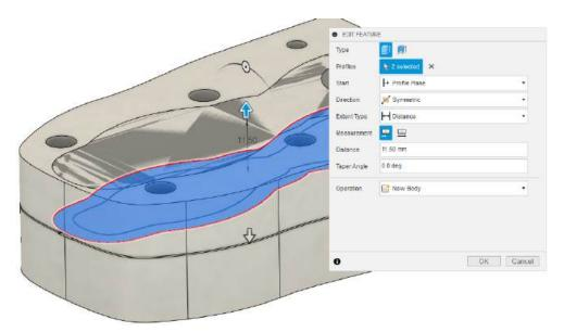
The next step involves using the <u>combine function</u> to integrate this simulation with the overall mould
