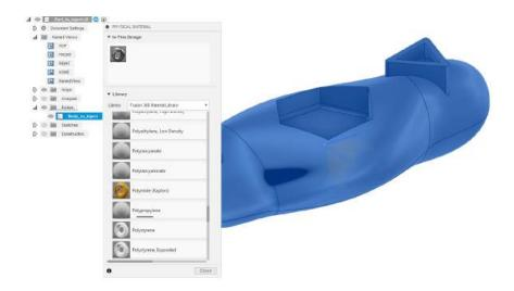
Once the physical material is set, the body properties can give the mass of the part.
