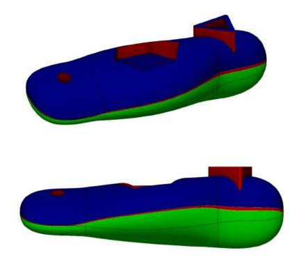
Analysing the silhouette of a part is crucial for mould design. It helps in understanding how the part can be demolded successfully without damage. In this case the silhouette line is tridimensional, schematised in red, separating the green from the blue.
