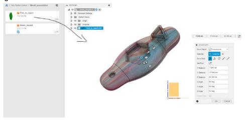
Utilise <u>the joint function</u> to position the imported 3D object by aligning it with the mould parting plane. Ensure the alignment of the demolding plane with the horizontal plane of the mould file.
