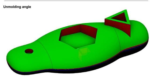
A minimum plastic moulding angle is required for demolding the part after injection. The analysis displays surfaces with a colour gradient based on the draft angle.
