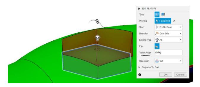
To change existing surfaces, using 3D parametric draft function
